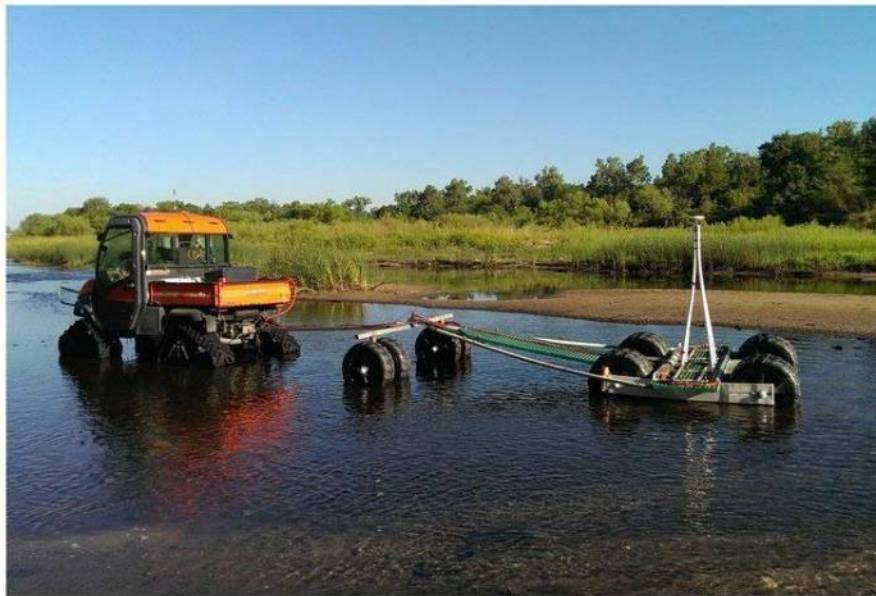
Figure 1-3. Shallow Water Digital Geophysical Mapping (Photo credit: 3DGeophysics.com)
