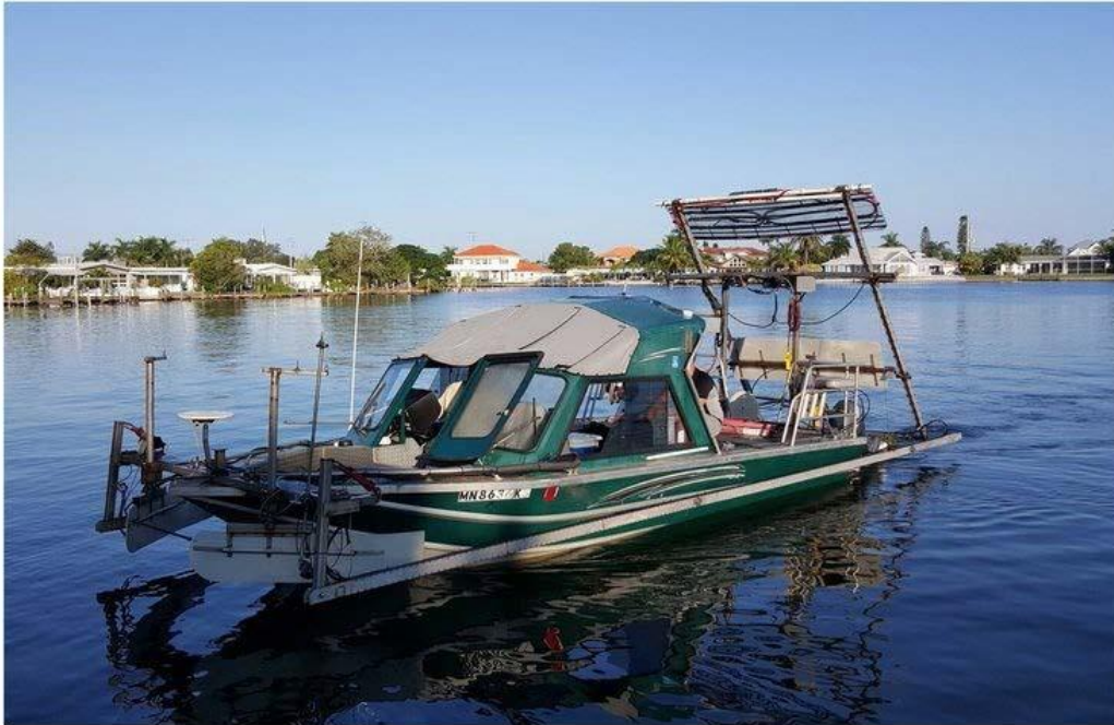
Figure 1-4. Deep Water Digital Geophysical Mapping (Photo credit: 3DGeophysics.com)
