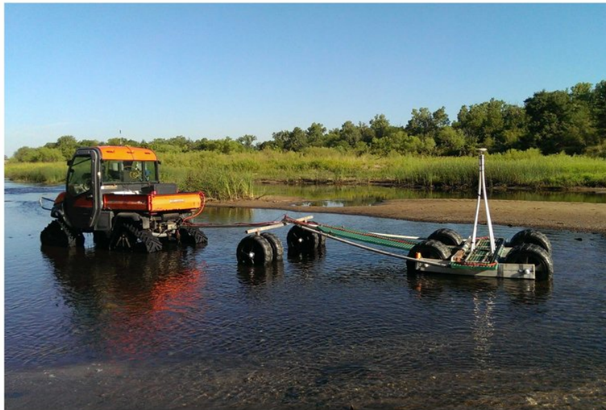
Figure 2.4-2. Surface digital geophysical mapping
